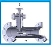
• **Steam-Atomizing Type:** Small amount of high pressure steam is used to atomize the cooling medium.
