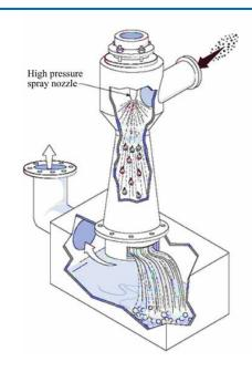
They use a change in gas velocity to shear liquid streams into tiny target droplets which particulate and soluble gases are transferred.
